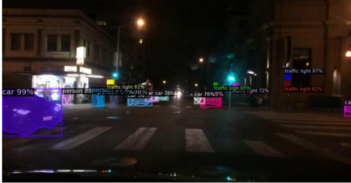
Figure 5. Detection, recognition and segmentation results for road objects in a BDD10K test image obtained by the Mask R-CNN model with Detectron2
