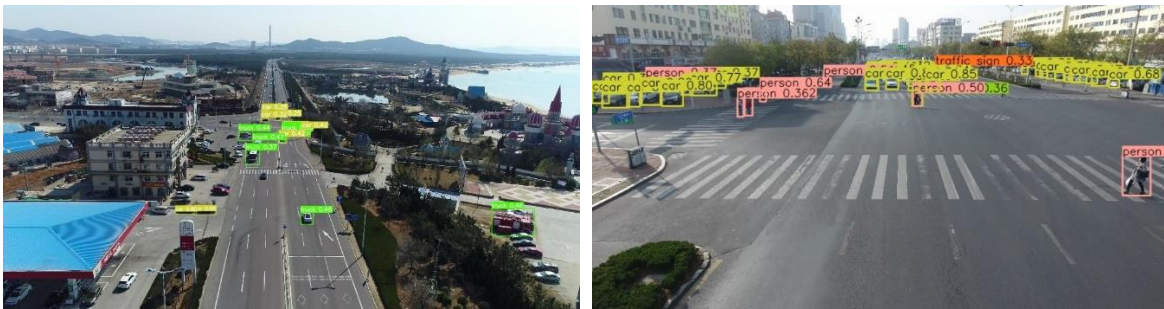
Figure 6. Road object detection and recognition results on two images from the UAVDT UAVDT_benchmark drone dataset obtained with our optimized model, showing the effectiveness of our model in detecting small objects.
