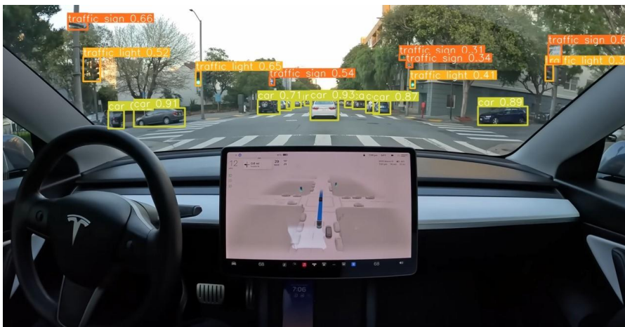
Figure 1. Example of result of road detection and recognition for a BDD10K-MV test image obtained with our optimized model.
